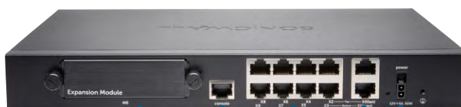
Expansion module Console port 8x1-GbE switch (configurable) X0 LAN port X1 WAN port Secure power
